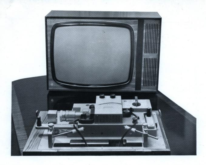
A teleplayer enabling unmodified Super 8mm film with magnetic sound stripe to be displayed on a domestic TV receiver or monitor. Known as the Vidicord, it uses conventional Super 8mm film, looks like a tape recorder, but feeds pictures via a cable into the aerial socket of a standard television set.
